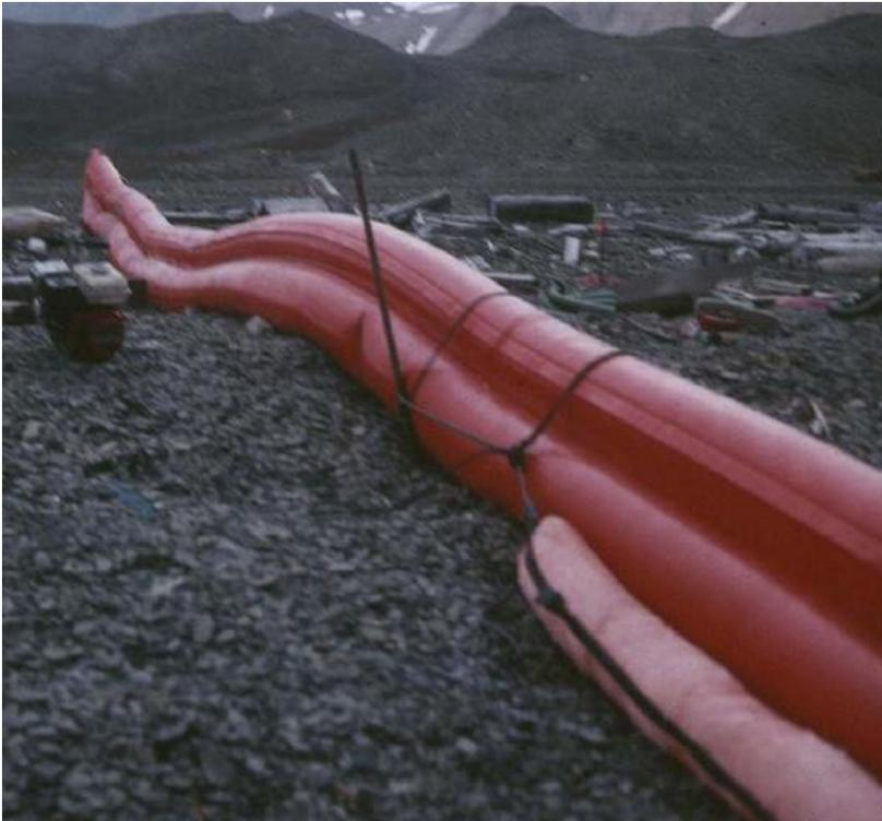
Water-ballasted (“shore-seal”) boom placed across the intertidal zone of a beach to prevent oil moving along shore. A length of sorbent boom (pink colored “sock boom”) is attached to the lower (intertidal) portion of the shore-seal boom (field trials on oiled beaches, Svalbard).
